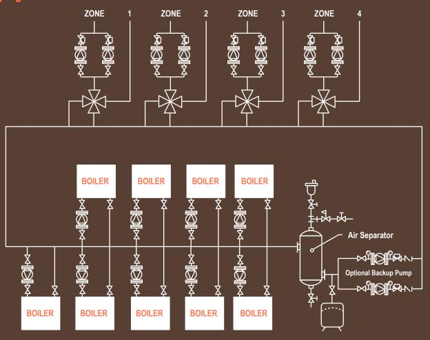
The boiler room is located at field level just inside the tunnel where Browns players enter the field. Nine Ajax Ace B15 Series 'G' boilers dominate the space like ready linemen. Each boiler is rated at 36 BHP and 1,500,000 Btu/hr, has a maximum allowable working pressure (MAWP) of 160 psi, and contains a patented, self-supporting copper fin coil. Safety relief valves are set at 125 psi with a relieving capacity of 1,700,000 Btu/hr.
